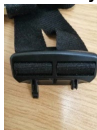
Broken prong on lanyard
