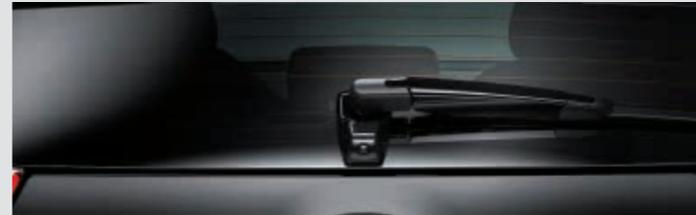
**Rear wiper-mounted rear camera** The rear camera is integrated with the rear wiper mount for a cleaner look, and to prevent lens soiling in bad weather.
