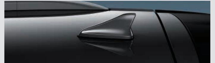
**Shark fin antenna** A stylish, aerodynamic shark fin antenna provides optimised reception for AM/FM radio, digital radio and navigation systems.
