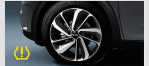
**Tyre Pressure Monitoring System (TPMS)** keeps track of the pressure inside each of the tyres. It tells you which tyre is reporting under-inflation by displaying its pressure value on the cluster screen.
