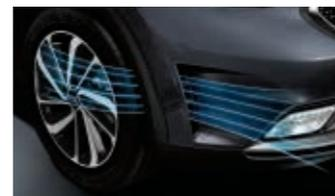
**Air curtain** An air curtain creates accelerated airflow at the front, reducing drag caused by turbulent air for improved aerodynamics.
