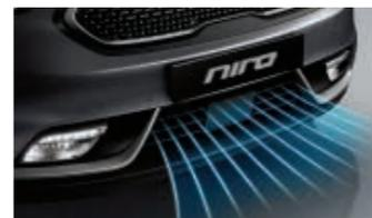
**Active air flap** An active air flap behind the grille cools the engine. It closes at higher speeds to reduce drag for better performance and fuel efficiency.
