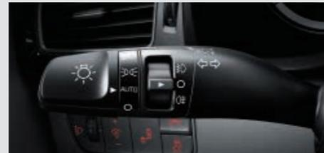
**Auto light control** Set the stalk control to auto and the headlights and tail lights will come on automatically at dusk or in dark places.
