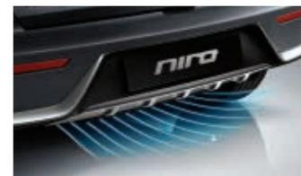
**Rear diffuser** A spoiler panel below the rear of the Niro is sculpted with longitudinal ridges for stability and aerodynamic control.
