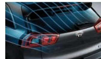
**Rear spoiler** Above the tailgate window, a rear spoiler takes advantage of airflow to help stabilise the body when travelling at speed.
