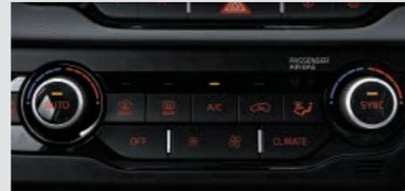
**Dual Full Automatic Temperature Control (D-FATC)** D-FATC automatically turns the air conditioner and heater on and off to maintain separate driver and front passenger temperatures (Self-charging Hybrid and Plug-in Hybrid).
