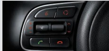
**Steering wheel mounted controls** Keep your eyes on the road. Remote controls let your fingertips adjust the audio, activate voice recognition, take or end calls, set speed limits and access the cluster menu.
