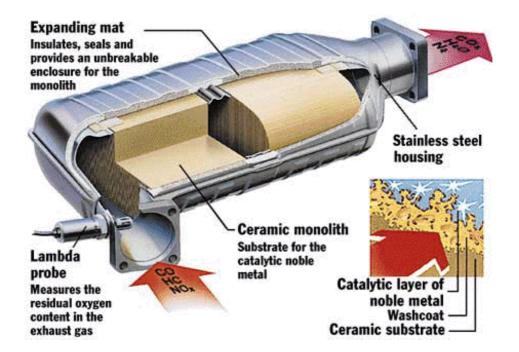
The use of catalytic converters leads to a dramatic reduction in the emissions of CO, HC and  $NO_x$ . However, they also result in an increase of  $CO_2$  emissions which do not cause a problem for urban air quality but do contribute to global warming.
